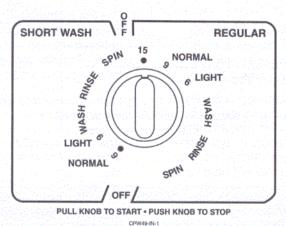
Pull the timer knob out to start the water fill. Agitation will begin when the water reaches the proper level.
